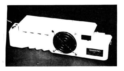
The **APPLEFAN** unit is an easy to fit accessory which reduces the risk of machine failures due to over heating when using certain interface cards.
